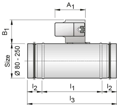
Controller structure and functioning as before, factory default setting, two-setpoint control via electric adjustment for an operating voltage of 24 volts, 50 Hz, as a two-setpoint controller with no intermediate position, Vmin and Vmax can be fixed by adjusting the mechanical travel stops.
